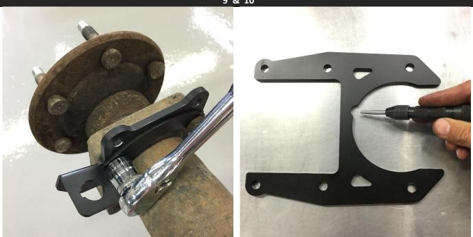
Bolt on the bracket parts as shown using the M12 bolts and washers to secure them to the axle flange (leaving them loose at this time). The same part will be attached to the bottom of the flange inversely, but without the hose bracket. Before installing the brackets, locate the notch as indicated. This will be mounted **UP** when the bracket is installed on the axle. Once installed, the brackets will position both calipers to the **REAR** of the axle.
